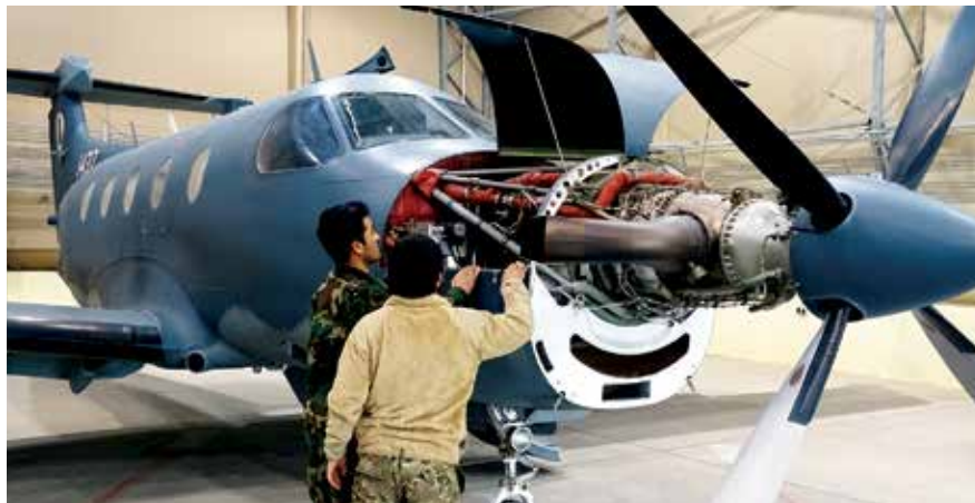
Special Mission Wing technicians examine a PC-12 aircraft during a scheduled maintenance inspection in Mazar-e Sharif. (NSOCC-A photo)
